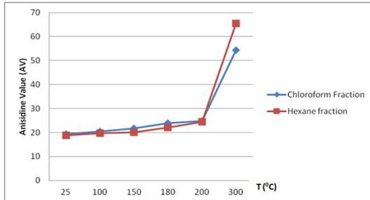
Figure 1. The anisidine value of red fruit oil (RFO) without antioxidant versus temperature (°C)
