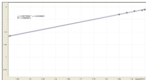
Figure 7. The calibration plot of FTIR-predicted anisidine value at region of 1685 - 1712 cm<sup>-1</sup> vs. actual value of AV of RFO as determined by IUPAC method in chloroform fraction.
