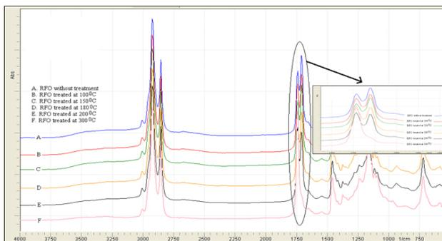
Figure 3. Absorbance changes in the region between 1650 and 1800  $\text{cm}^{-1}$  of the infrared spectrum of RFO under elevated temperature.
