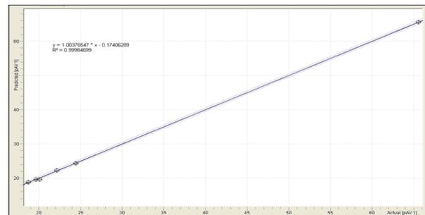
Figure 6. The calibration plot of FTIR-predicted anisidine value at region of 1685 - 1712  $\text{cm}^{-1}$  vs. actual value of AV of RFO as determined by IUPAC method in hexane fraction
