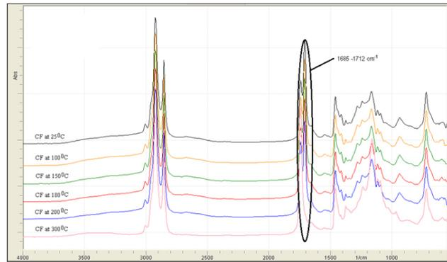
Figure 5. ATR FTIR spectra of RFO in chloroform fraction under elevated temperature condition. Region assigned with circle were selected to develop anisidine value (1685 - 1712  $\text{cm}^{-1}$ ) in the calibration model.
