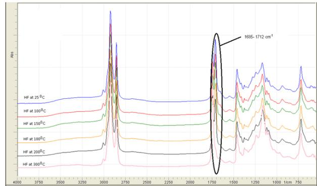
Figure 4. ATR FTIR spectra of RFO in hexane fraction under elevated temperature condition. Region assigned with circle were selected to develop anisidine value (1685 - 1712  $\text{cm}^{-1}$ ) in the calibration model.
